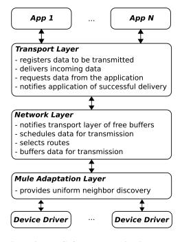
Figure 3. The CafNet communication stack.
