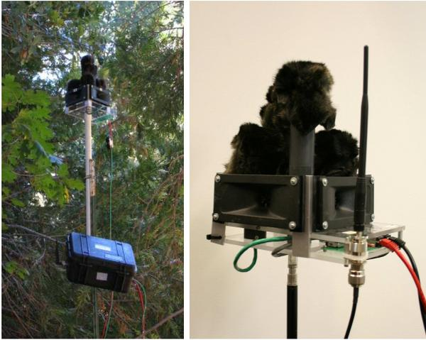
Fig. 2. The Acoustic ENSBox Platform.
